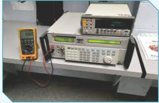
Fluke Multiproduct Calibrator with 300 MHz Oscilloscope (Model: 5502A-3), Fluke 6.5 Digit Digital Multimeter (Model: 8846A). Fluke 50 Turn Current Coil (Model: 5500A/Coil).
